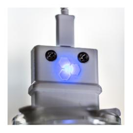
In normal operation, while it is dispersing silver ions into <u>distilled water</u>, the **SILVERengines** *proton* will be slowly and calmly blinking blue.
