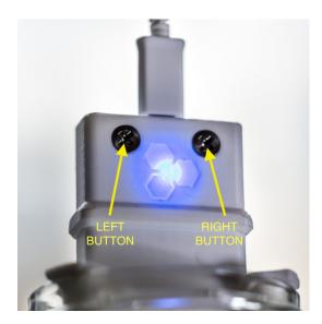
There are two stainless steel screws on the front of your **SILVERengines** *proton* that serve a dual purpose. They not only hold the **SILVERengines** *proton* assembly together, they are also the controls by which you can set the **SILVERengines** *proton* to one of its five available levels of <u>ionic/colloidal</u> <u>silver</u> solution strength.
