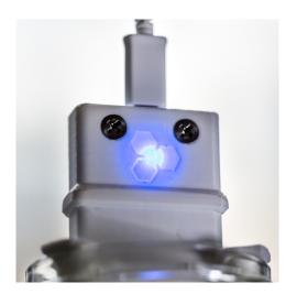
In normal operation, while it is dispersing silver ions into <u>distilled water</u>, the **SILVERengines** *proton* will be slowly and calmly blinking blue.
