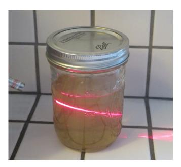
For fun, shine a red laser pointer through pure <u>distilled water</u> before you process it - you should not see a "beam," though perhaps you'll see "sparklies", i.e. little flecks of dust.
