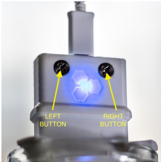
There are two stainless steel screws on the front of your SILVERengines *proton* that serve a dual purpose. They not only hold the SILVERengines *proton* assembly together, they are also the controls by which you can set the SILVERengines *proton* to one of its five available levels of [ionic/colloidal silver](#) solution strength.
