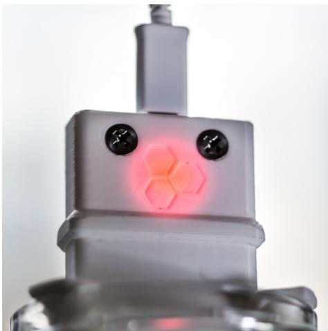
When your **SILVERengines *proton*** is starting up, it quickly tests to be sure that you are using pure, [distilled water](#) by measuring the conductivity of the water.
