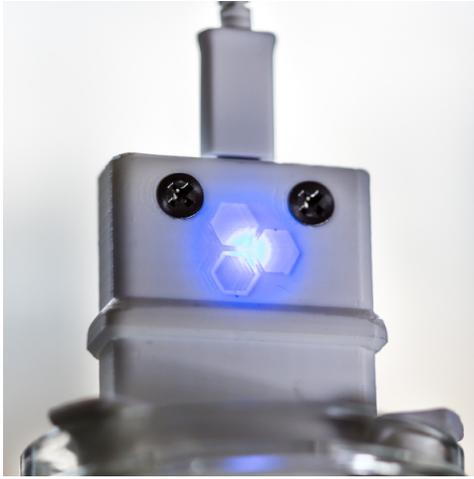
In normal operation, while it is dispersing silver ions into [distilled water](#), the **SILVERengines *proton*** will be slowly and calmly blinking blue.
